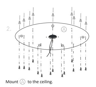
Note: When mounting be sure to locate and mount  $(\underline{\mathbb{A}})$  to a joist/celing beam
